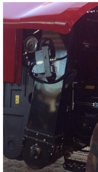
When the grains have been measured, the sample is released into the downside of the clean grain elevator and is returned to the grain tank. Samples are measured every 7-12 seconds or around every 15meters down the row as the combine strips the grain. The protein, moisture and oil data are displayed on the Touch Screen PC mounted inside the cabin. Figures 2, 3 and 4 show three screen shots for the various options to display the data.
